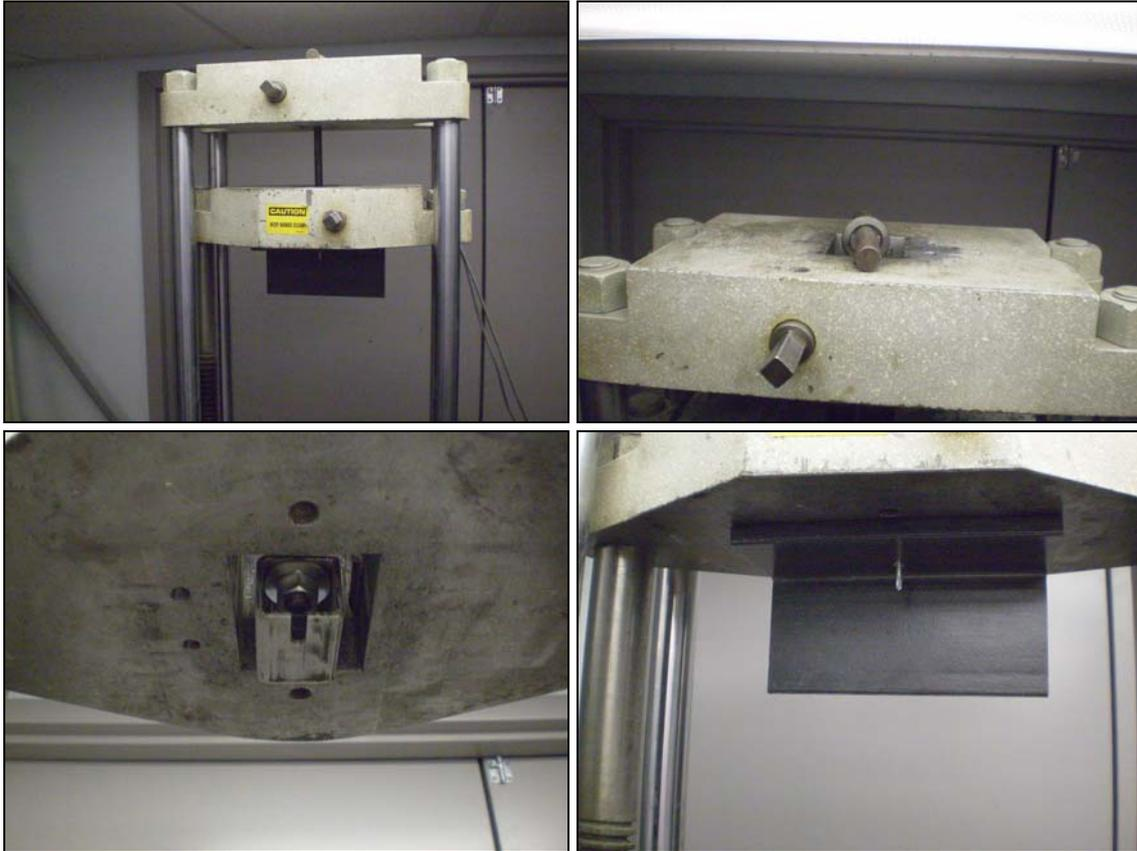
Figure 2. Pull-out strength test fixture and set-up.
