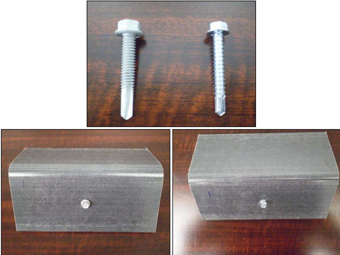
Figure 1. Fasteners and samples before testing (1/4 - 20 fastener left, #12 - 14 right).
